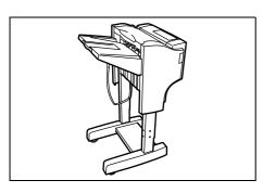
The document finisher holds a large quantity of finished copies. The finisher offers a convenient means of sorting. Sorted finished copies may also be stapled. For further details, refer to the Document Finisher *Operation Guide*.
